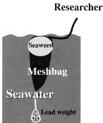
Fig. 31 Schematic diagram showing how to measure the density of seaweed.
